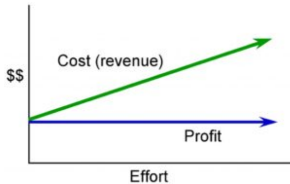
Figure 13.2: In a cost-reimbursable or cost-plus contract, the contractor is guaranteed a fee, but the client's costs can increase based on effort.
